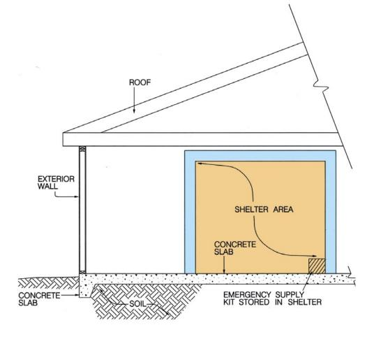
susceptible to the impact of missiles, it should not be built of wood framing. Instead, it should be built of concrete or concrete masonry. Access to this type of shelter can be provided through an existing door or window in an exterior wall of the house.
