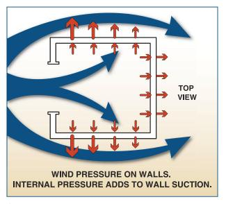
Figure II.1 Effect of extreme winds on building roof and walls
