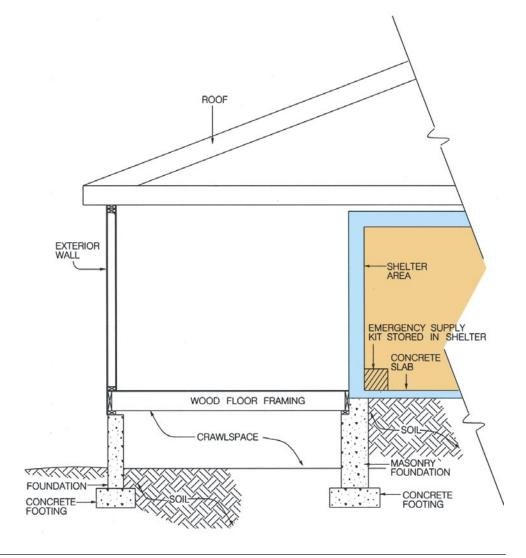
be separate from the framing of the house. As shown in Figure II.4, a shelter built inside the house cannot use the floor of the house. The shelter must have a separate concrete slab floor installed on top of earth fill and must be supported by concrete or concrete masonry foundation walls. An alternative approach, which may be more economical, is to build an exterior shelter on a slab-on-grade adjacent to an outside wall of the house and provide access through a door installed in that wall.
