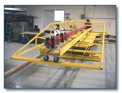
Missile (debris) launcher, Wind Engineering Research Center (WERC), Texas Tech University carried by extreme winds. The shelter designs in this booklet account for these findings by specifying building materials and combinations of building materials that will resist penetration by missiles in extreme winds.
